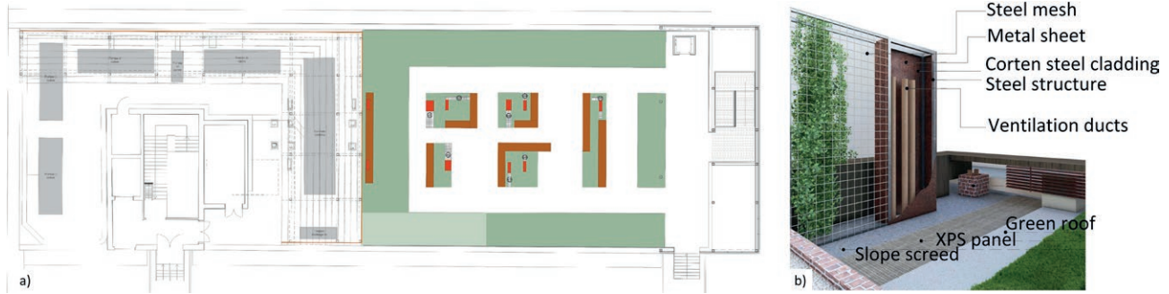
Figure 9. From left to right: a) roof plan: on the right, the accessible area highlighted in color; on the left, the service zone dedicated to mechanical systems; b) mitigation system for drainage columns and internal ventilation units, along with the roof assembly and stratigraphy. (Source: Authors).
