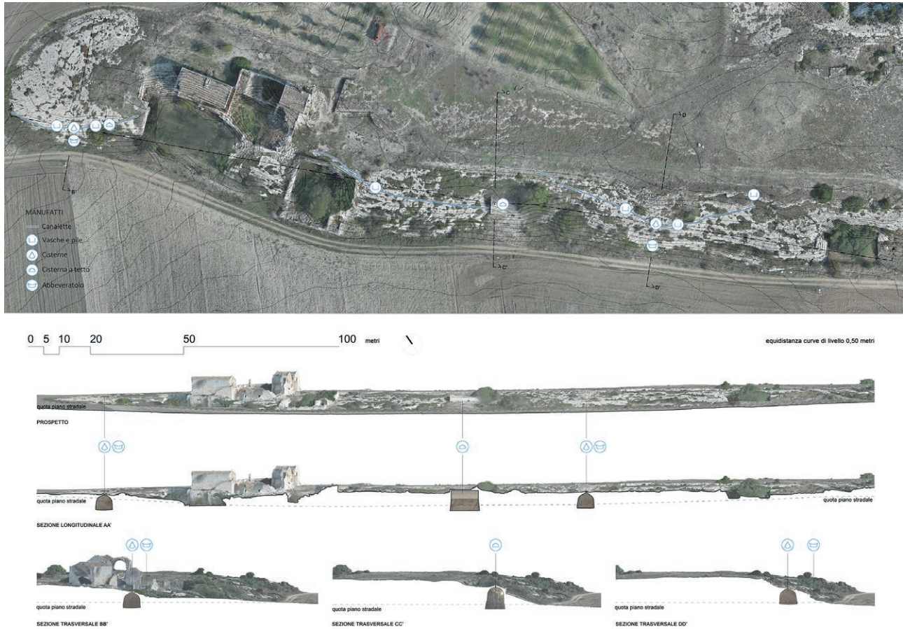
Figure 3. Plan, elevations and sections of the integrated water resources management system and analytical graphs of the interception, channeling, collection and use subsystems. © 2025, Daniele Altamura, Enrico Lamacchia.
