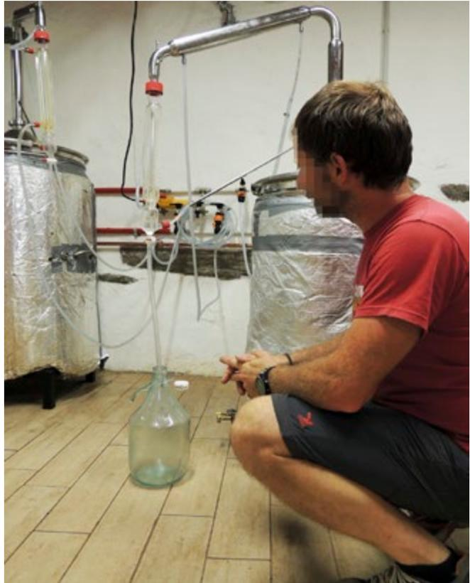
**Fig. 4 and 5.** Modern alembic at work. The distillation cycle starts with the flowers heated, in order to produce oil and distilled water. Both are placed into a 1lt bottle. They are separated only after some days. The essential oil is put into small size bottles.
