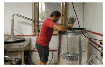
**Fig. 4** and **5**. Modern alembic at work. The distillation cycle starts with the flowers heated, in order to produce oil and distilled water. Both are placed into a 11t bottle. They are separated only after some days. The essential oil is put into small size bottles.
