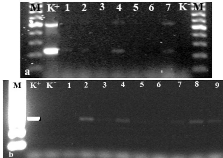
Figure 2. Gel electrophoresis analysis of polymerase chain reaction products amplified by duplex-PCR (a) and RG-PCR (b) performed on individual cones of the *columellae* of fruits. K<sup>+</sup>, bacterial suspension (10<sup>8</sup> cfu mL<sup>-1</sup>) of *Pseudomonas syringae* pv. *actinidiae* CRA-PAV 1530; M, molecular marker (100 pb DNA Ladder Plus; Fermentas, Lithuania); K<sup>-</sup>, negative control (water).
