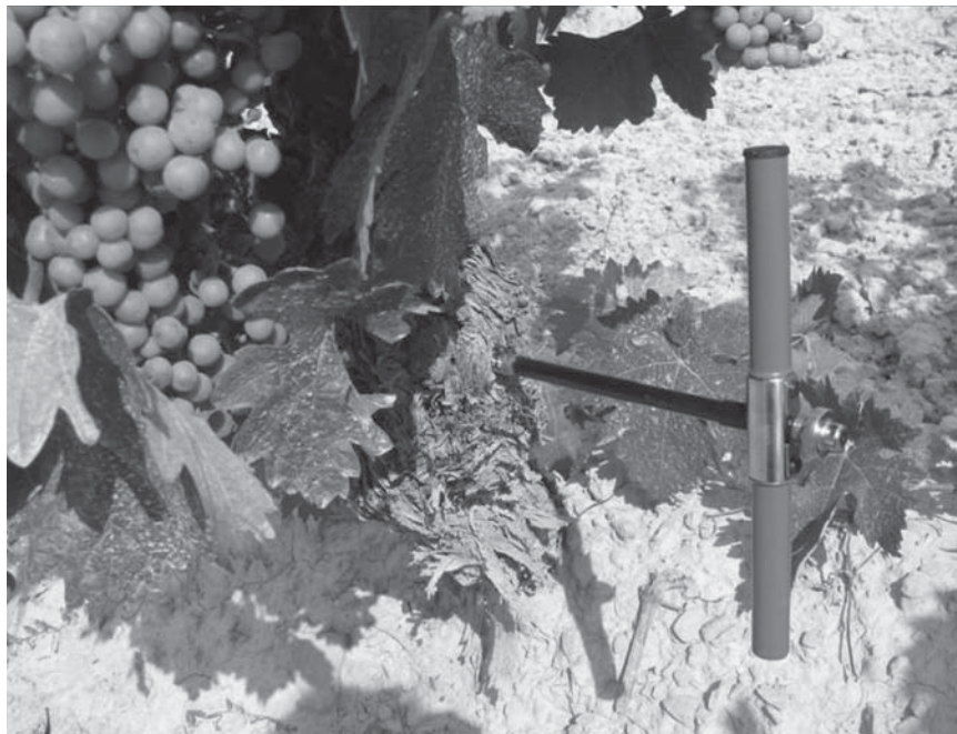
Fig. 1. Sampling of grapevine wood by means of an increment borer.
