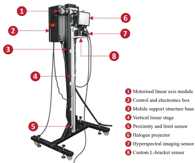
Figure 2. Phenotyping platform for hyperspectral image acquisition using vertical scanning of plants. The platform consists of a mobile support structure, a motorized vertical linear-stage module, a dedicated lighting system, a hyperspectral imaging sensor mounted on a custom bracket, and a control and electronics unit. Videos of the platform in operation during hyperspectral data acquisition are available in the CSIC institutional repository at https://doi.org/10.20350/digitalCSIC/17945 .
