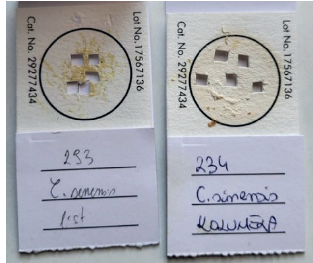
Figure 4. FTATM Classic Micro cards (Qiagen) printed with leaf (left) and fruit (right) tissues of a sweet orange tree infected with CLBV than had fruit creasing and leaf blotching symptoms. Cut-out pieces were used for optimization of the protocol for detection of CLBV by extraction-free RT-PCR. The photo was taken two months post printing.
