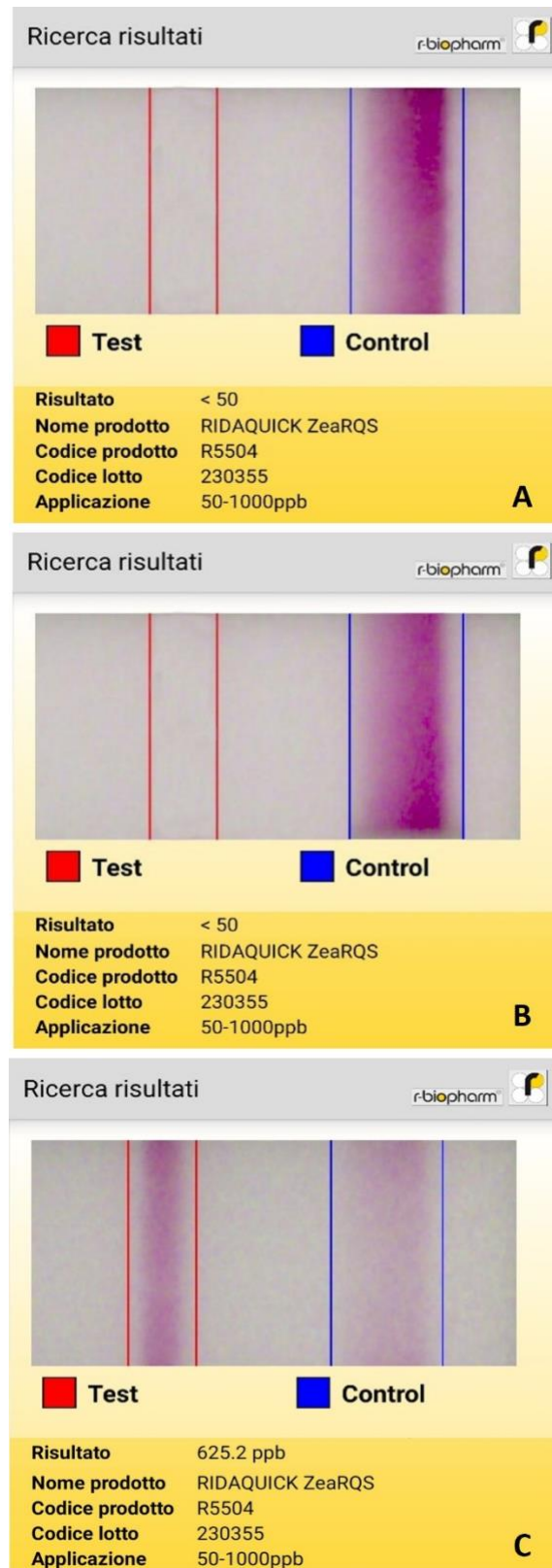
Figure S5. The output of the RIDA® QUICK Zearalenon RQS test kit. Results are acquired using the RIDA® SMART APP. A) Mock control; B) Fusarium oxysporum isolate DAFE SP21-23; C) F. pseudograminearum isolate 3B.
