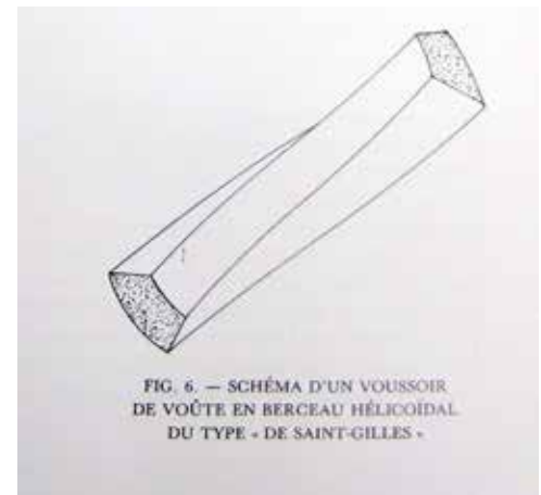
Fig. 12 Schematic drawing of a stone in a screwed barrel vault in the manner of the spiral stair case of Saint-Gilles (by A. Hartmann-Vimich, 1996).
