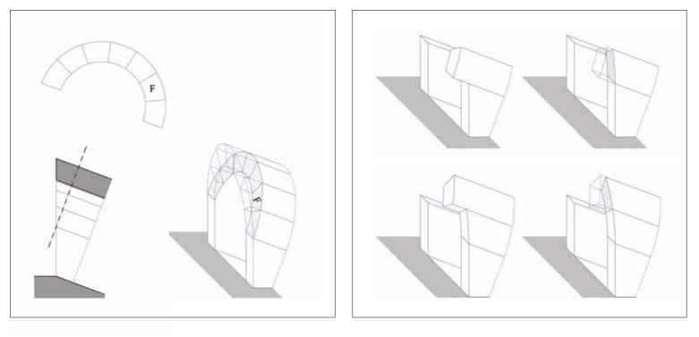
Fig. 9 Longitudinal cross-section, transversal cross-section and axonometric view of the entrance to a descente de cave (drawing S. Galletti).
