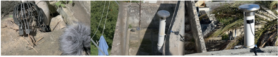
Figure 15. Kitchen terrace. Left: microphone positioned next to the water pipe. Right: contact microphone mounted on the chimney connected to the boiler.
