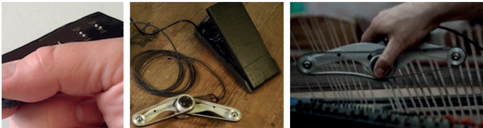
Figure 5. Paul Vo's Wond includes a haptic feedback system to provide a sense of touching the string. Léo Maurel's Archet Motorisé (right) a motorized wheel bow with variable speed via a foot pedal.
