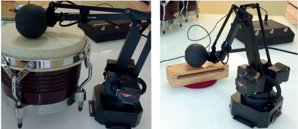
Figure 6. uArm desktop robotic controlled via Leap Motion performed several sounds for Qualia. Also, it has been used to perform timbre maps, as part of the Fab synthesis project, for woodblock at a 0.5mm distance per strike. The woodblock experiment gave 35500 sounds at 355 x 100 strikes across its surface.
