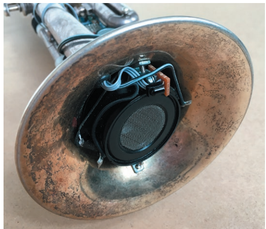
Figure 11. Speaker in bell, with IR detector at top.
