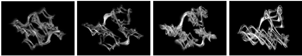
Figure 3. Transition of the space curve going from a waveform with odd to all harmonics (left to right). The odd-harmonic space curve has three perpendicular planes of 2-fold improper rotation ( S_2 ) symmetry.
