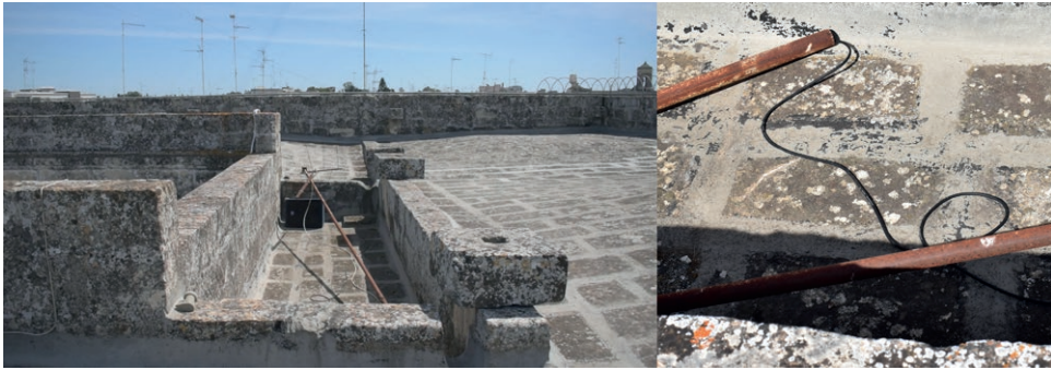
Figure 13. Collettore. Left: view from the West rooftop. Right: detail of the old antenna, with microphone inserted in the tube.
