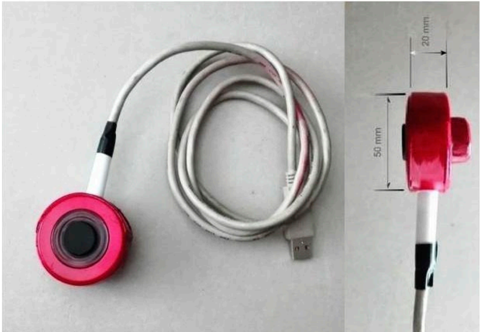
Figure 1 – . PRD electronic dynamometer.
