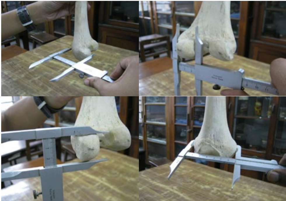
Figure 1 – Measurement of different morphometric parameters of femoral condyles by Martin's sliding caliper.
