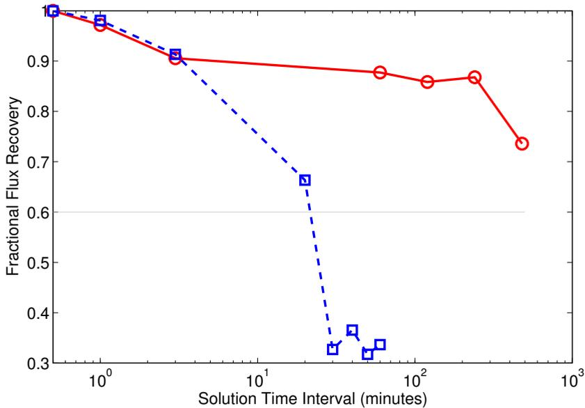
Figure 2. Coherence timescales at 130-GHz for FTP data (blue dashed) and SFPR data (red solid). This is to be compared to the coherence times at 130GHz of ~tens of seconds. The FPT correction alone provides a hundred-fold improvement in coherence time.
