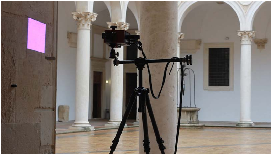
Figure 6 – The GOM system during data acquisition
