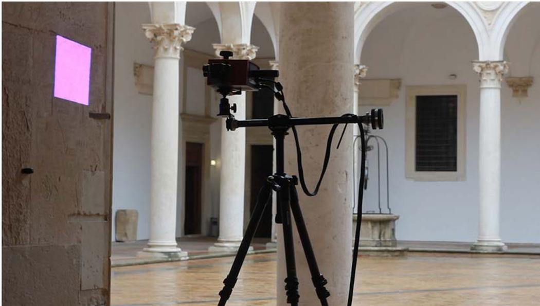
Figure 6 – The GOM system during data acquisition
